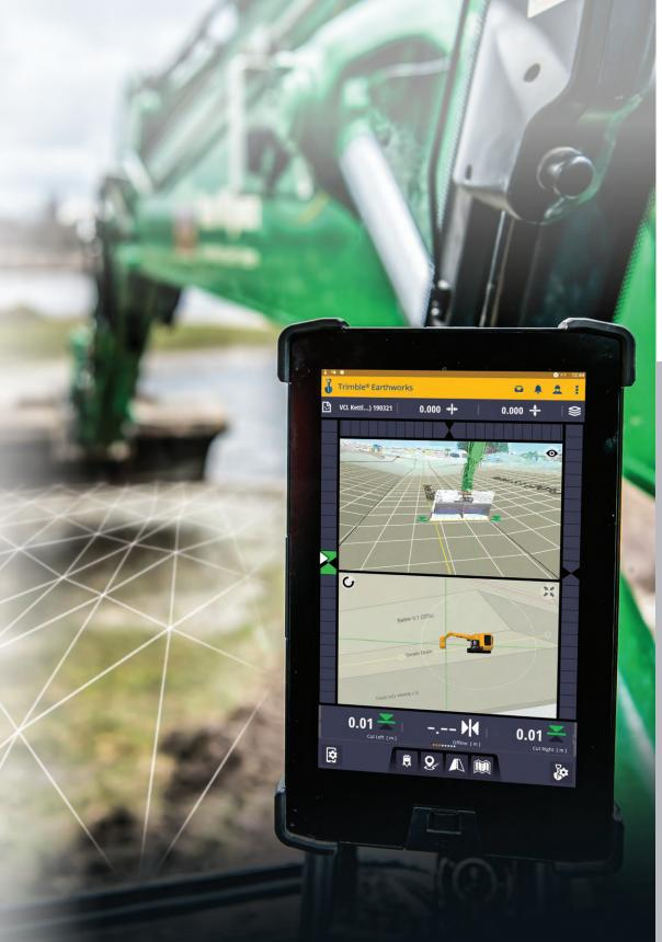
**2D CONFIGURATION FOR HEIGHT AND SLOPE** - Flexible starter solution for excavation, canal and trench construction, grading and profile work — the start of productivity.
