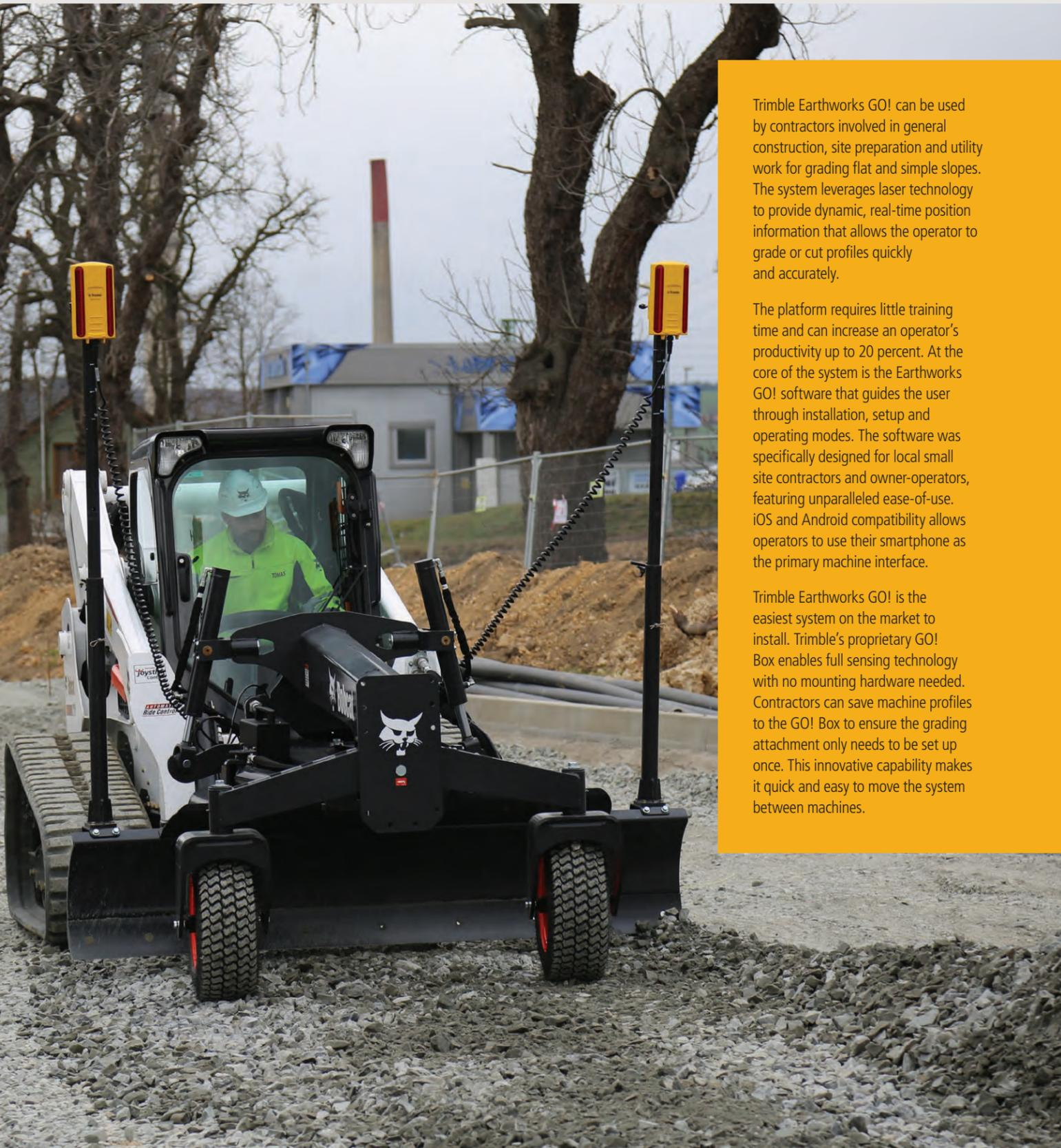
Trimble Earthworks GO! can be used by contractors involved in general construction, site preparation and utility work for grading flat and simple slopes. The system leverages laser technology to provide dynamic, real-time position information that allows the operator to grade or cut profiles quickly and accurately.
